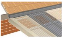
UNDER A GUTTER - Fit back channel flashing with foam infill strips under gutter prior to laying sheets and metal barge capping to edge of sheet.
