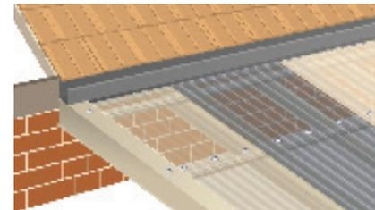
UNDER A GUTTER - Fit back channel flashing with foam infill strips under gutter prior to laying sheets and metal barge capping to edge of sheet.
