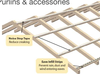
1. Ensure that your roof pitch is at least 5°, ie. 88mm rise per lineal metre. This will ensure adequate water run off.
