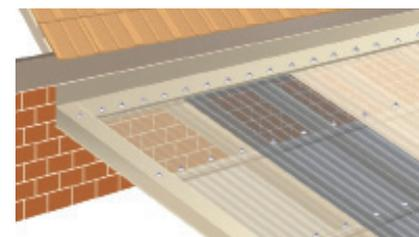
AGAINST A WALL/FASCIA - Fit metal barge capping to edge of sheet and metal apron flashing at the wall or fascia.
