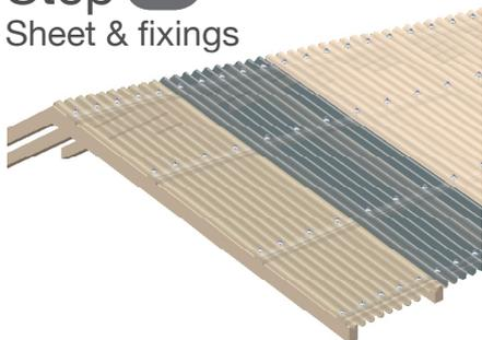
1. Ensure that the UV surface protected side faces the sun. This is the side of the label and the inkjet marking. When installed as a wall or fence it is recommended that the UV protected side is facing the most sun. The life of the sheet may be shortened and discolouration may occur due to the unprotected side being exposed to UV radiation.
