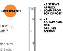
Assemble posts by screwing them back to back with 7 staggered screws.
